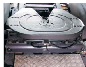
Practical example, fifth-wheel support plate: usually 6 lube points
